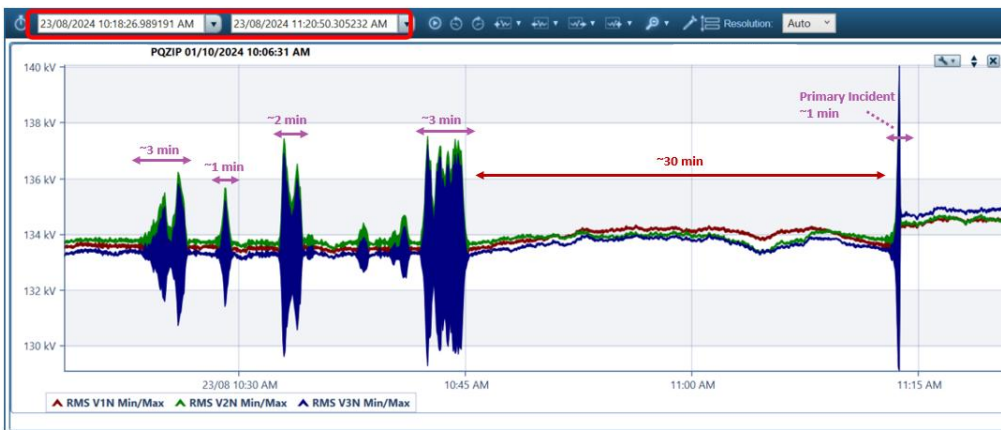
Figure 2 Multiple voltage oscillations in EC on 23 August 2024 prior to Primary Incident
