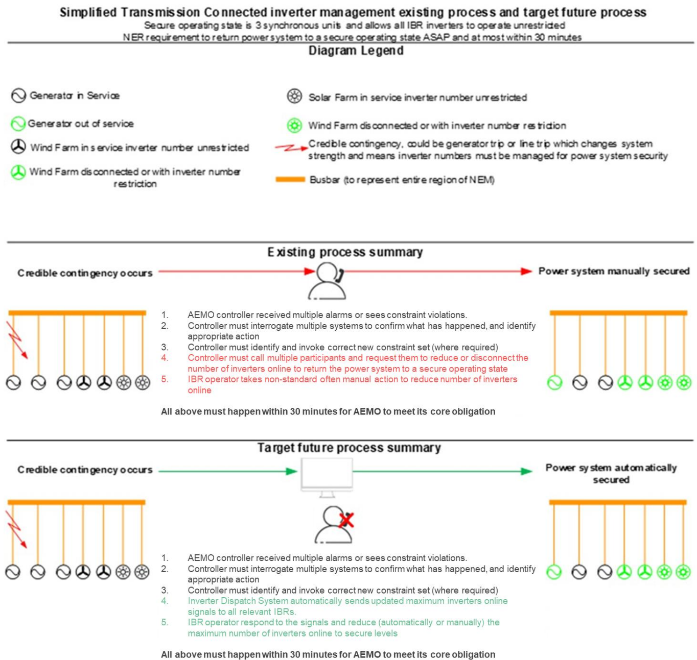
Figure 2 Inverter management current and target future state summary, in a credible contingency scenario
