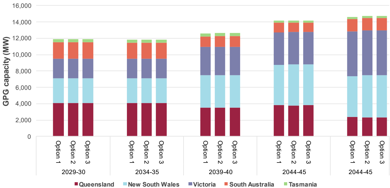
Figure 14 Forecast GPG installed capacity across different plausible gas development projections, Step Change, 2029-30 to 2049-50 (MW)
