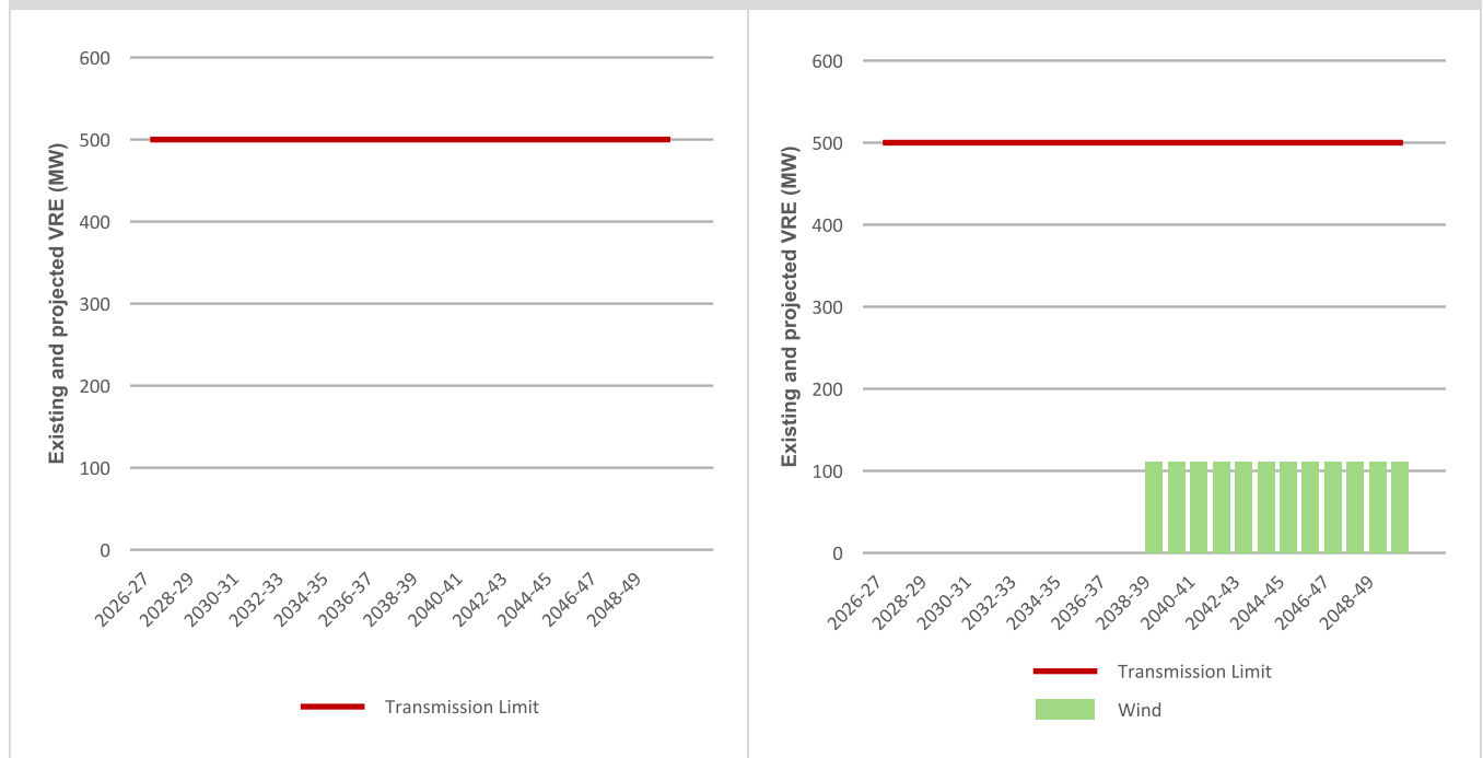
Transmission access expansion forecast for Slower Growth (left) and Step Change (right)
