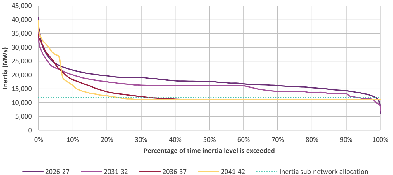
Figure 18 Projected levels of inertia available in Victoria, Step Change scenario (MWs)
