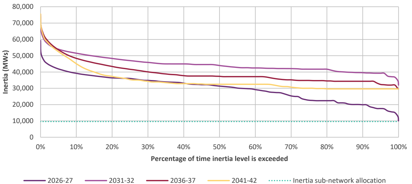
Figure 6 Projected levels of inertia available in New South Wales, Step Change scenario (MWs)
