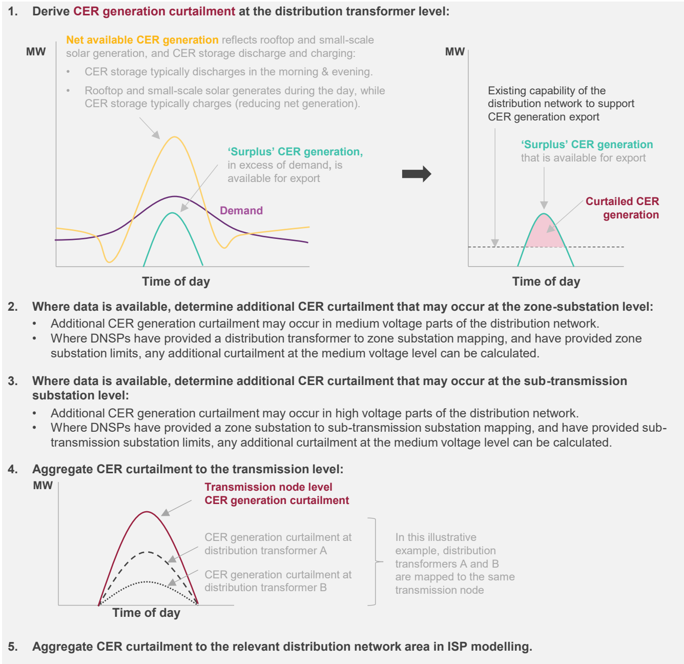
Figure 5 Illustration of the CER curtailment modelling under the LV Asset Data Template Pathway
